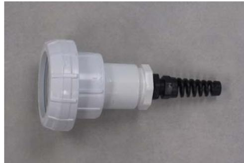
The camera housing incorporates simple nylon and PVC components that press fit together, or utilize threaded compression fittings to connect to one another. Note, all fittings that press fit require PVC cement to seal against water incursion.
