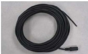
**The camera cable** is the component of the system designed to carry power down to the camera module and the video signal back to the surface. The black PVC jacket of the camera cable provides a watertight layer surrounding the individual conductors of this cable, while the 3.5mm female stereo plug provides an ideal means of connecting the camera to the surface-mounted components.
