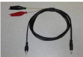
**The power/video adapter cable** is the component of the system designed to distribute the conductors of the camera cable between the topside power source and a suitable video monitor.
