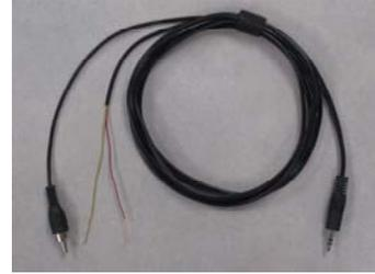
41) Using the #26 AWG wire stripper, strip approximately 3/4" of insulation from the ends of the individual wires. Be careful not to cut any of the copper conductors within the insulation.
